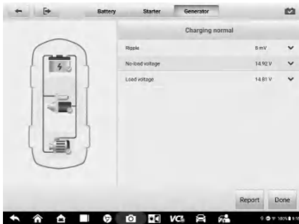
Figure 13-8 Generator Test Results Screen
