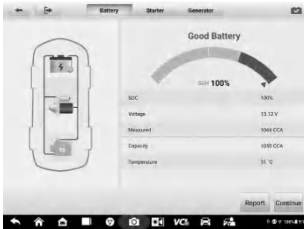
Figure 13-6 Battery Test Results Screen
