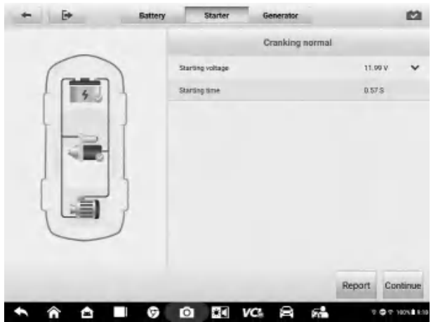
Figure 13-7 Starter Test Result Screen
